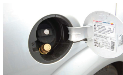
Figure 2. Liquid petroleum gas (LPG) supply valve, in the fuel cap compartment.
