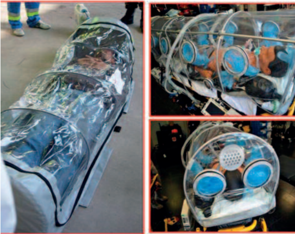
Figure 6. Negative pressure isolation capsule with HEPA filter.
